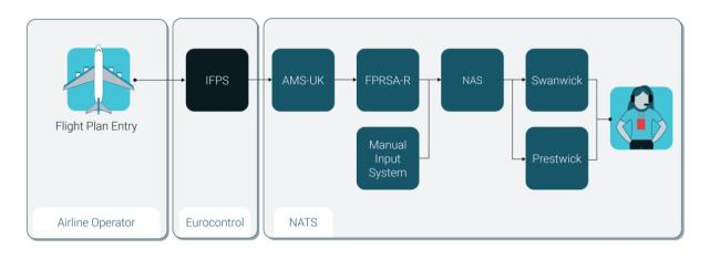
FPRSA-R has a primary and backup system monitored both by dedicated Control and Monitoring (C&M) systems and also an aggregated central C&M system.
